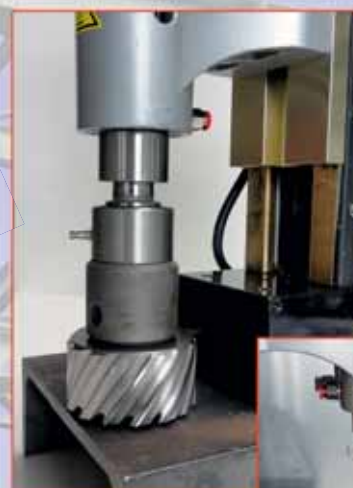
Kernbohren / Core drilling
